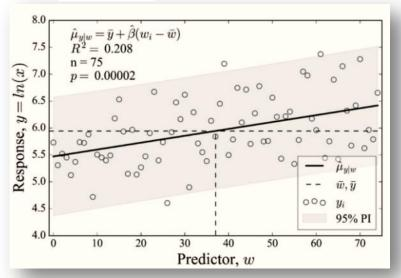
**Fig. 1.** Natural logarithm y, of annual maximum streamflow *x* of the Aberjona River at Winchester, MA, 1940–2014 versus w = time in years. Solid line is a bivariate linear regression which represents the conditional mean of  $y = \ln (x)$  as a function of *w*, denoted  $\hat{\mu}_{y|w}$  Shaded region is the estimated 95% prediction interval for future values of  $y = \ln (x)$ .
